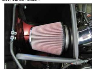
21. Install the K&N® air filter onto the filter adapter and secure with the provided hose clamp.
