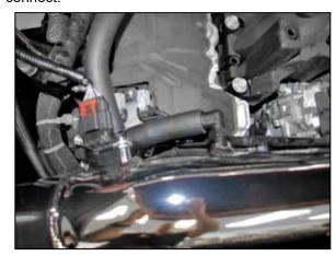
20. Using the provided vent hose, connect the factory vent to the 90° fitting installed into the K&N® intake tube. Reconnect the mass air sensor electrical connection.
