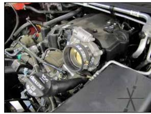
16. Install the provided coupler (08186) onto the throttle body and secure with the provided hose clamp.
