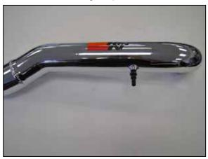
14. Install the quick connect fitting into the  $K\&N^{\circledcirc}$  intake tube as shown.
