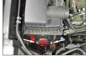
6. Remove the two nuts securing the air filter housing to the inner fender and then remove the housing from the vehicle.
