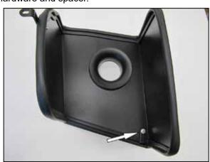
10. Install the provided heat shield mounting bracket (070015) onto the heat shield using the provided hardware and spacer
